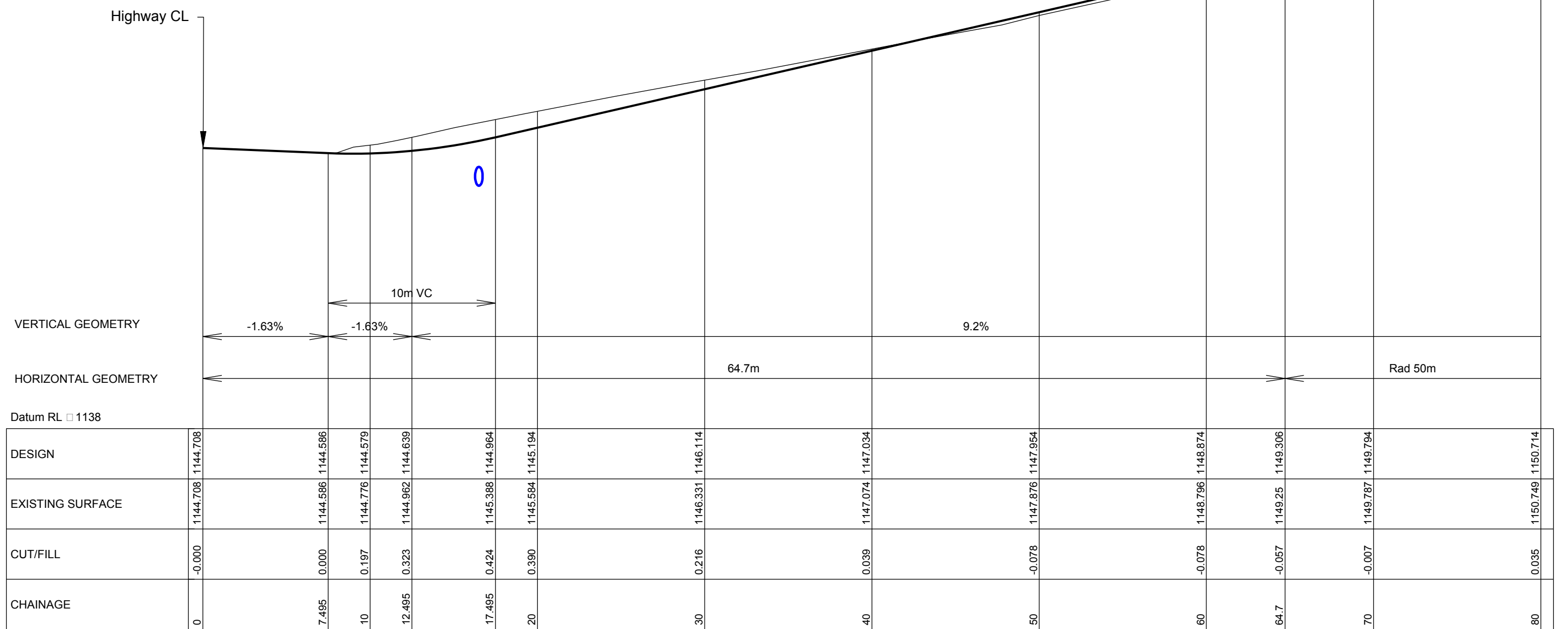
LONGSECTION: WINDFARM ACCESS ROAD CENTRELINE
